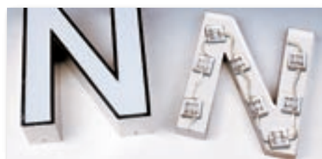
NOTE: When mounting in channel letters, depth of channel should be at least 4 cm deep to prevent "hotspots" of light from LED modules.
