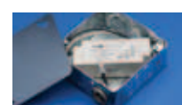
LED SH-24-20W-HW 20 W hardwire, maximum 2 pcs of 18 LED fixtures, 4 pcs of 12 LED fixtures, 8 pcs of 6 LED fixtures OR any combination up to 48 LEDs Input: 100 – 240 V AC Output: 24 V DC 4 1/8" x 4 1/8" x 1 1/2" (120mm x 58mm x 38mm)
